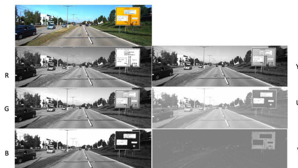
Figure 3: Schematic diagrams of the image after the separation of the RGB & YUV channel. The left column is the set of RGB channel separation images, and the right column is the set of YUV channel separation images.
